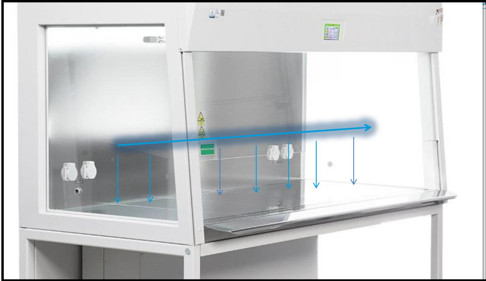
***Smoke shall be passed from one end of the cabinet to the other, along the centerline of the work surface, at a height of 4 in (10 cm) above the top of the access opening.***
