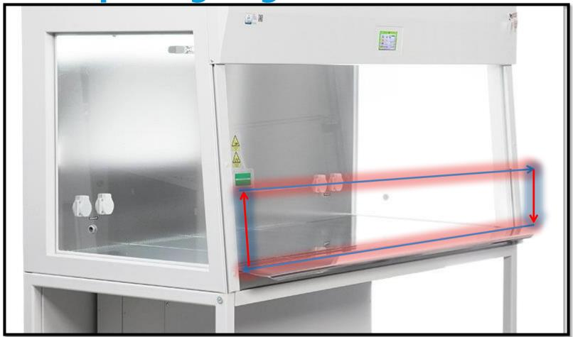
Smoke shall be passed along the entire perimeter of the work opening edges, approximately 1.5 in (3.8 cm) outside the cabinet. Particular attention should be paid to corners and vertical edges.
