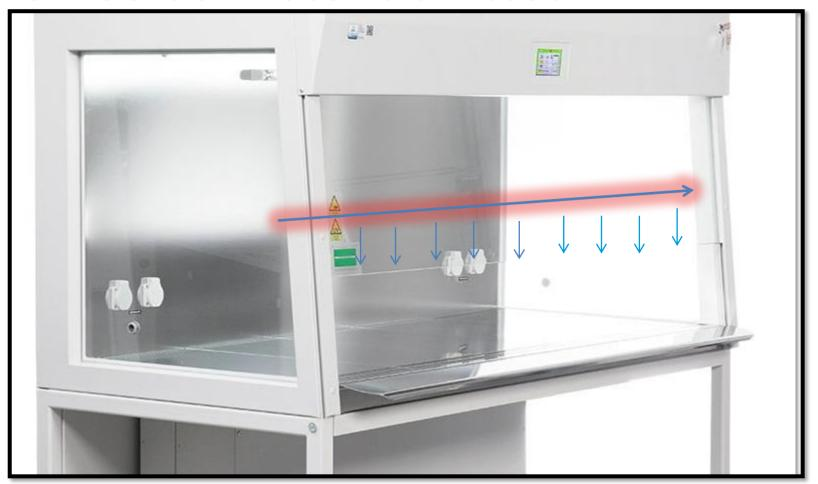
Smoke shall be passed from one end of the cabinet to the other, 1 in (2.5 cm) behind the view screen, at a height 6.0 in (15 cm) above the top of the access opening.
