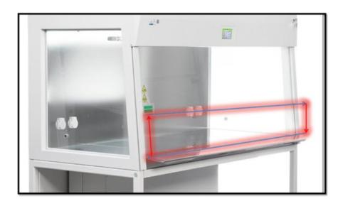
Smoke shall be passed along the entire perimeter of the work opening edges, approximately 1.5 in (3.8 cm) outside the cabinet. Particular attention should be paid to corners and vertical edges.
