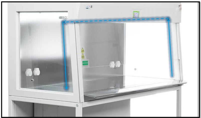
Smoke shall be passed up the inside of the window 2 in (5 cm) from the sides and along the top of the work area.
